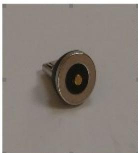
*Photo 3: Magnetic Power Cable Adapter*
