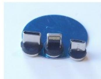
*Photo 2: Mag Cable Adapters - C and Lightning and Micro*
