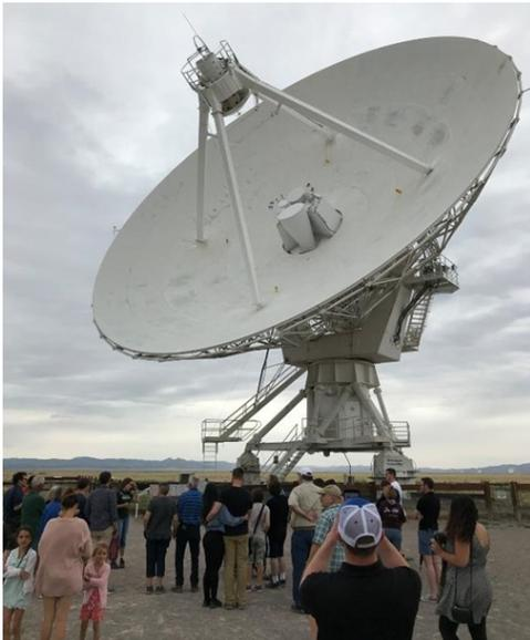
Each leg of the “y” formation contains nine disks, which can be rearranged in several ways. The configuration changes periodically from fully spread out along the “Y” to fully compressed and to two intermediate designs. The effect is to widen the aperture of the telescopes or to narrow them.
